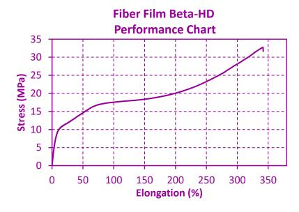
The graph above illustrates how the film performs under an increased load. Where the line ends indicates where the film breaks.
